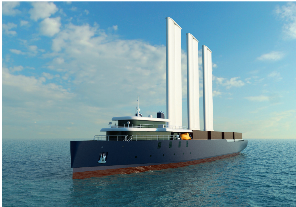
Zephyr & Borée propose a freighter powered by rigid sails which consumes 30% less fossil fuel.
